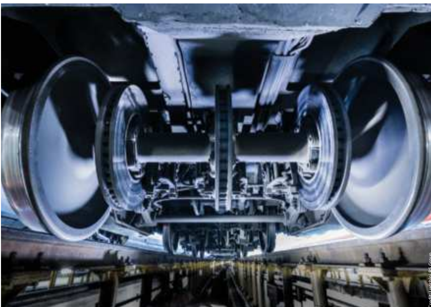
Wheelsets with noise absorber panels assembled on an ETR1000 bogie
