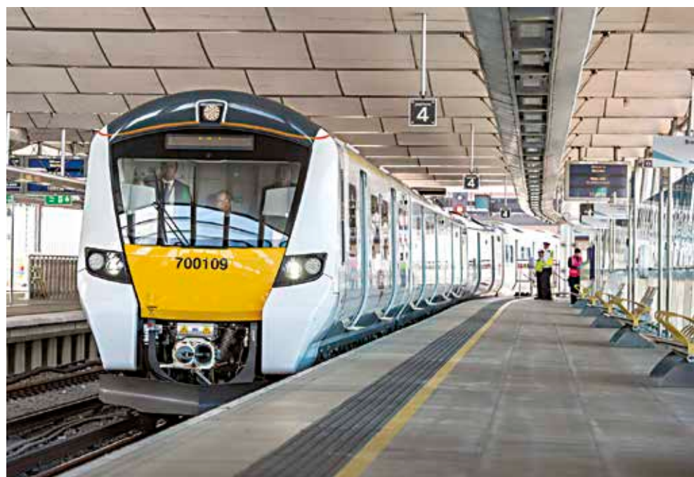
A Siemens Class 700 EMU began test running through London in December using the ATO over ETCS Level 2 being installed as part of Network Rail's Thameslink Programme.
