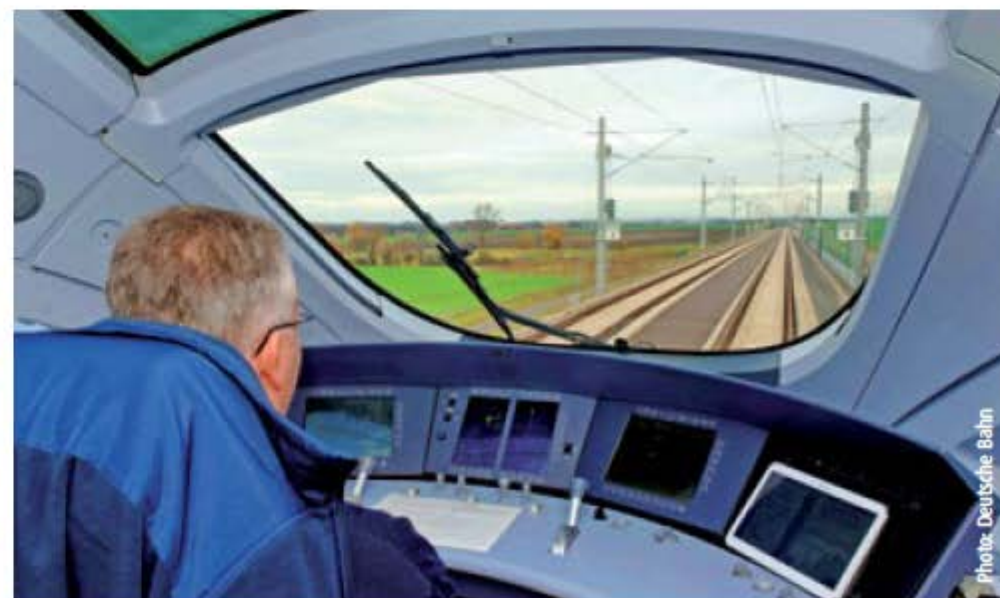
ETCS Level 2 equipped trains are guided by cab signalling.
