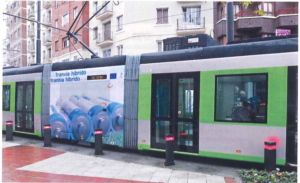
A CAF tram fitted with an on-board energy storage system was tested in the Spanish city of Vitoria-Gasteiz.
