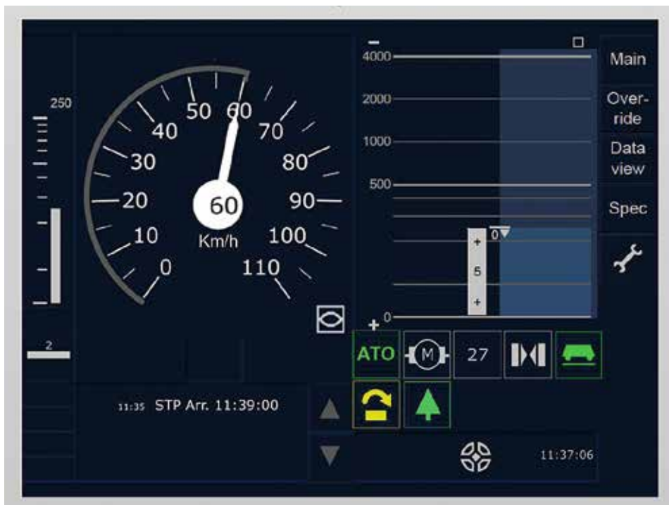
Using the AoE interface specifications, both ATO and ETCS information can be displayed to the driver on the same DMI.
