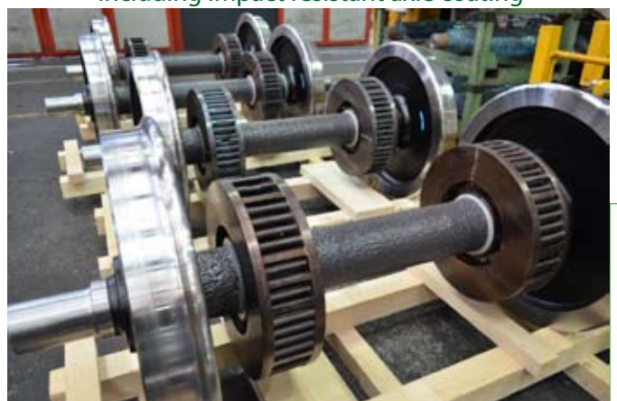
The SUSTRAIL wheelsets including impact resistant axle coating
