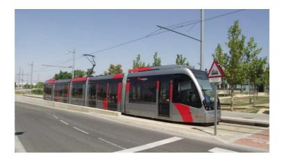
In 2009, a year after the city's successful hosting of Expo 2008, a team of companies was contacted to build a new tramway in the city. The first phase of the system was built using onboard energy accumulation technologies that enable lower energy consumption and head wire-free operation in some sections of the city centre. It opened in 2011.
